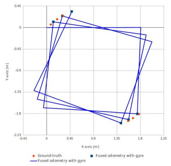
This graph shows the position error of fused odometry with gyro, when robot moves along a square path. Robot moved with 0.1 m/s on the line segment and rotated with 30 deg/s on the corner.
