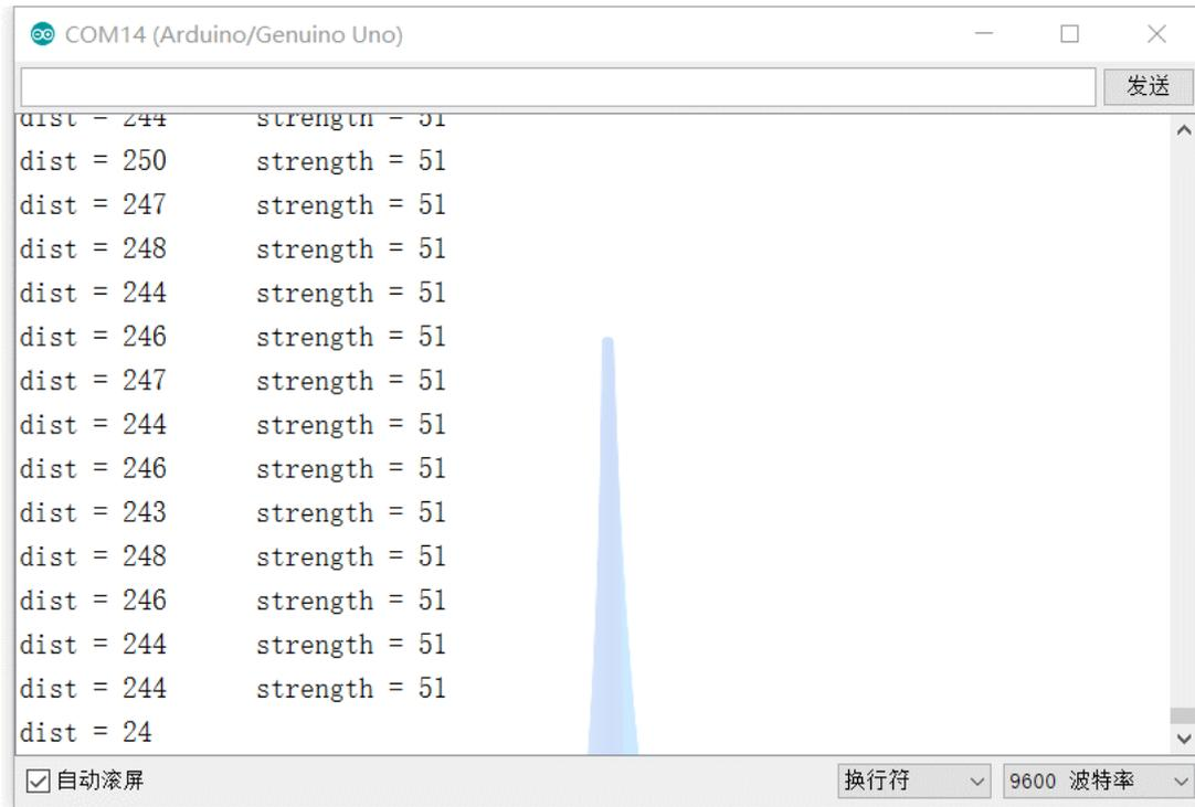
Figure 3. LiDAR Data Displayed on Serial Monitor
