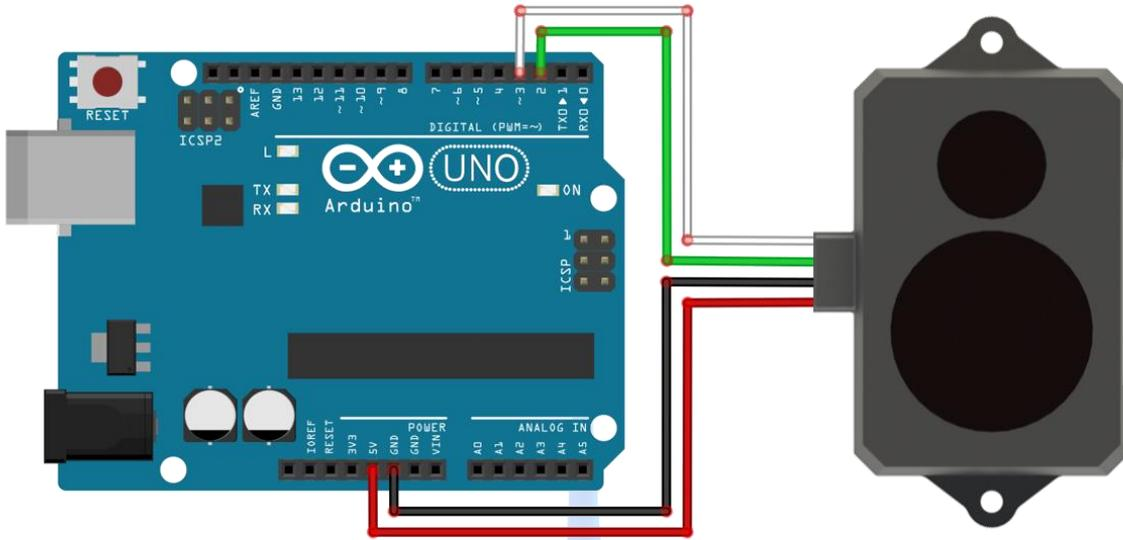
Figure 1. Wiring Diagram for TF02 and UNO Board
