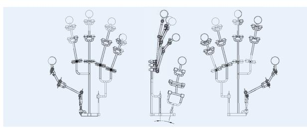
9 electric motors control the motion functions in 20 joints
